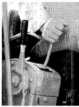
Hydraulic blade control levers engage smoothly and crisply. Response is immediate and always predictable regardless of engine RPM, or with two or more levers engaged at once. Variable displacement piston pump senses hydraulic system needs and automatically adjusts hydraulic flow. Closely spaced levers and short travel engagement reduce operator effort.
